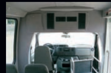
Standard 45,000 BTU/HR passenger heat and air conditioning mounted above driver to maximize passenger area head room in rear of bus
