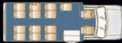
138" W.B. 21' 14 Passenger with Co-Pilot and Cargo Space
